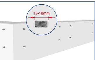
3. Attach backing to the wall and adjust to get more alignment(6-12mm), then fixed by washer and nut.
