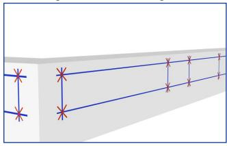
2. The bolts to be chemical fixed into wall leaving 15-18mm out of the wall for nut and pin.
