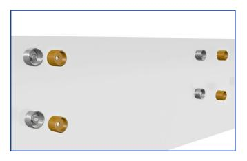
5. Fit bodies(with plastic bush) by winding in, suggest around 2mm off wall.
